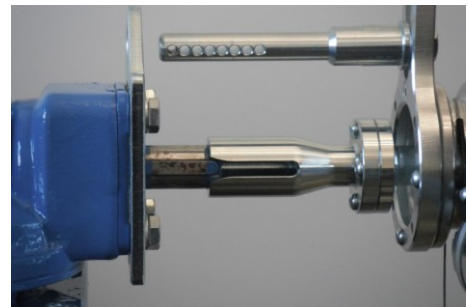
3. Connection of the APB/APS to the gearbox shaft
